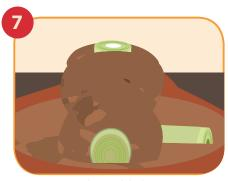
Start putting mud around the banana stem in the middle, make sure to press hard or else the stove will break easily. Keep adding mud until the whole stem is covered.
