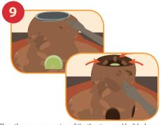
Place the saucepan on top of the the stove and build a layer of mud around the saucepan. Make all the sides stove smooth. You can use a knife or pang. Also put 3 pan supports holders inside. This is where your saucepan will sit. After 5 days, pull out the saucepan and the 2 banana stems on the side.
