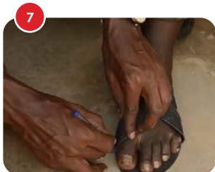
7 Measure the jeans fabric straps on your sandal model to determine the space needed for the foot. Using a pen, mark where the fabric meets the sandals.
