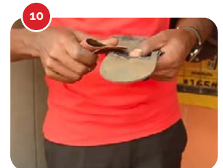
10 Use sandpaper to smoothen the surface. Use the sand paper also to remove dirt on the car tire inner tread material
