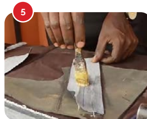
5 Carefully apply glue on the edges and on the middle line of the fabric.
