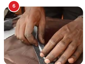
6 For each of the 4 straps, fold the right and left edge to meet the middle line.
