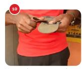
Use sandpaper to smoothen the surface. Use the sand paper also to remove dirt on the car tire inner tread material
