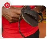
Trim off the excess rubber from the sandal using the blade. Use sandpaper to gently smooth out the edges.
