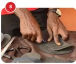
Use a cutter blade to create openings where the marked points are.
