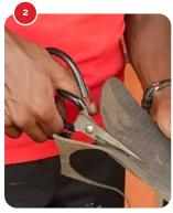
Carefully trim off the excess layer following the line of the pen. Do the same for the car tyre inner tread material (or rubber piece).
