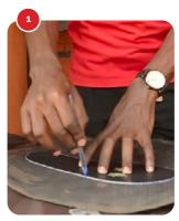
Place the foot size patterns on the cow-mat layer (or rubber piece) and trace with a pen.
