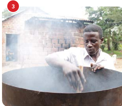
Continue burning the organic waste to make a charcoal-like carbon-based material. Keep mixing all the waste to ensure that it all burns. 3
