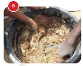
Add clay soil into the water and cassava mixture to form a thick paste.7
