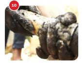
Smear a little of the cassava solution that was set aside into the mould and place the carbonized material into the mould to form briquettes.9
