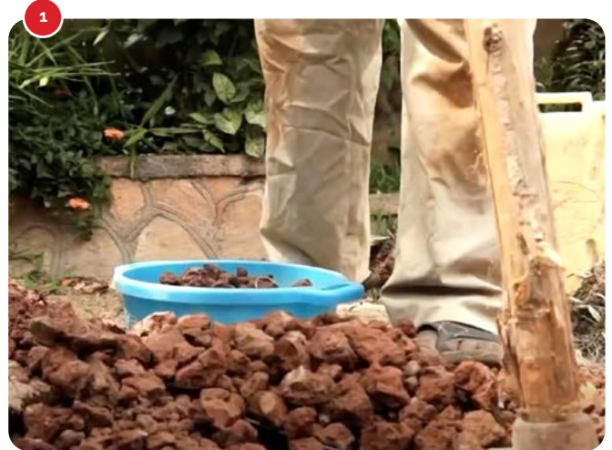
1 Get clay soil and break it into small pieces. Use clay soil from an anthill.
