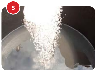
5 When the CMC has dissolved, add in the 2 teaspoon spoons of caustic soda and stir thoroughly.
