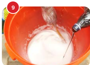
9 Once foam is formed, add in ½ kg of sulphonic acid and stir to dissolve.
