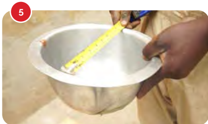
5 We mold the top of the stove basing on the size of a sauce pan. Select a saucepan and measure its inside width in centimeters using a measuring tape. For this example, we used a saucepan that was 21cm wide. 2
