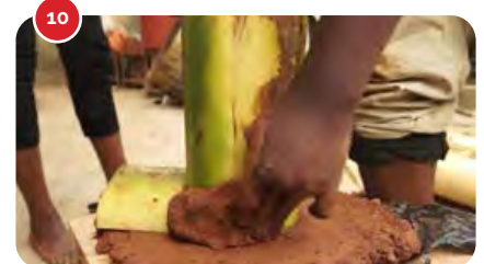
10 Get the banana stem cuttings for the air inlet (smallest cut part) and for the main stove chamber (uncut banana stem) and place it on the base. Start molding the clay soil mixture around the banana stems.
