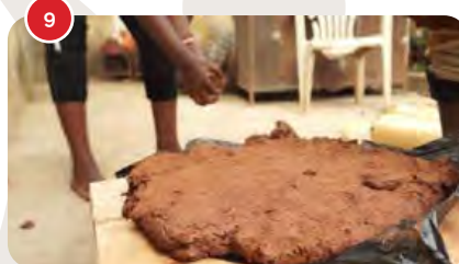
9 On a flat surface, mold a stove base determined by the saucepan size. At the base is where we put our strength because it is the foundation of our stove Note: Use recycled polythene bag to lay on the wood before starting to add soil so that it does not stick to the surface.
